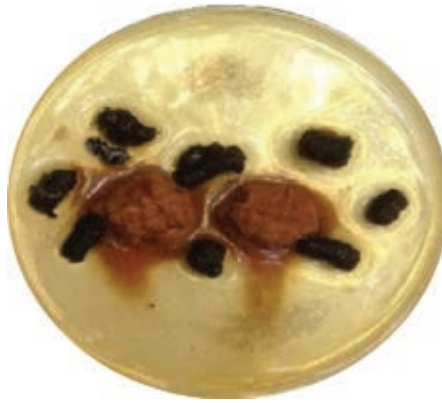
Fig 2. Same dispersive clay treated with Peats TailorMade™
